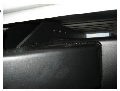
Insert the factory jounce stop bolt into location to ensure the bracket will not fall during installation. Do not torque this bolt down. It will be tightened further along in the installation process. See figure to the Right
