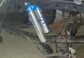
3.6 Install Shock Absorber Bolts and Nuts
