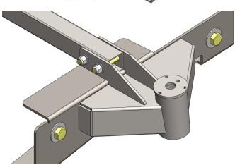
Torque OE jounce stop bolt to 32 Foot-Pounds (13mm tools) and use a thread locking compound.
