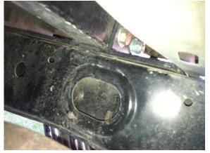
Start with the passenger side rear frame support mounting bolt hole. Insert the wrench into the cutout and align the flange nut with the frame support mounting bolt holes. See Figures below
