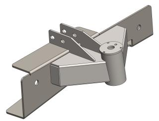
Place the support up onto the frame and align the cross tube in between the cross tube mounts. see figure to the Right
