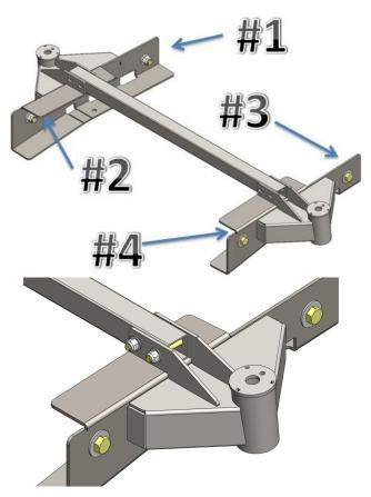
3.3 TORQUE Cross Beam Hardware
