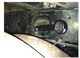
Locate one of the 3/4" -10 x 1.75" Bolts and a large washer. (1 1/8" Tools) Insert the bolt into the hole and thread the bolt into the flange nut. If you drop the nut, don't worry, simply use a magnet to retrieve the flange nut. Prior to torquing down the bolt and nut, you want to get the remaining 3 started. Follow the sequence to the Right. Torque bolts to 250 Foot-Pounds.
