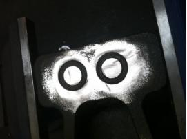
Locating center of the Pin on the OE block. Measure the Diameter of the locating pin. Divide the value by 2. Scribe a line as shown. Scribe an additional line at 90 Degree intervals to find center of the pin
