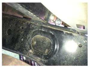
Start with the passenger side rear frame support mounting bolt hole. Insert the wrench into the cutout and align the flange nut with the frame support mounting bolt holes. See Figures below
