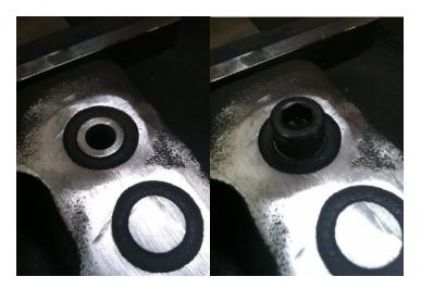
Place Socket Head Cap Screws (SHCS) into Block. Insert the 1/2" washer with the 1/2"-13 Ny-Lock Nut on the inside of the block.
