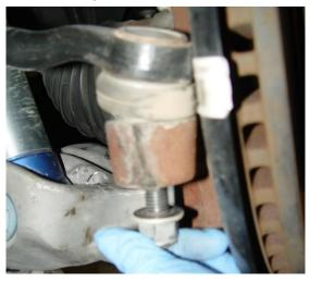
To Loosen, Tap on Knuckle and bottom of ball joint with Hammer
