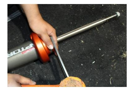
\*\*\*\*\* USE A COUPLE ZIP TIES TO KEEP LIVE VALVE WIRE FROM GETTING TANGLED IN THE COIL SPRING \*\*\*\*\*\*\*\*\*
