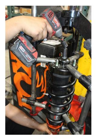
Remove shock absorber from coil spring
