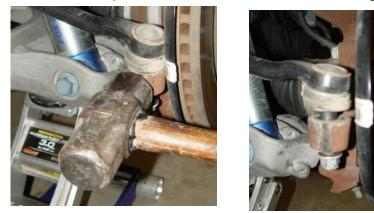
• Upper Control Arm to Knuckle Attachment Stock Upper Control Arm to knuckle ball joint. Remove this using the same method as the OE stock Tie Rod. 18mm Nut
