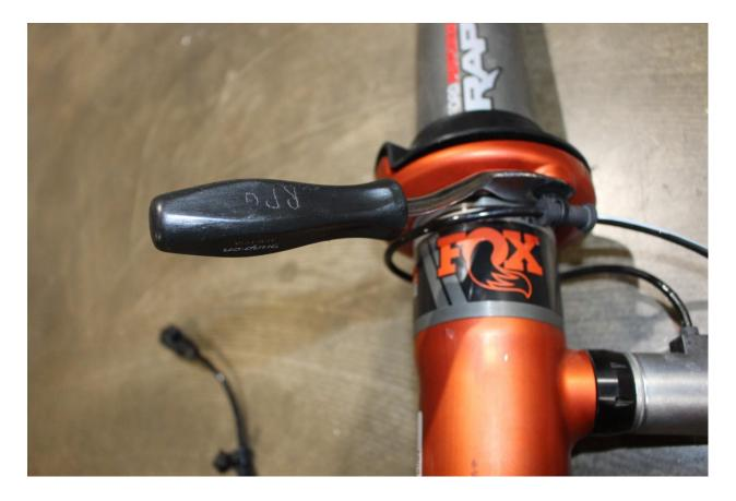
Slide up coil spring perch to expose retaining rings. This may require a soft hammer, be careful to not damage the aluminum.
