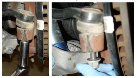
To Loosen, Tap on Knuckle and bottom of ball joint with Hammer
