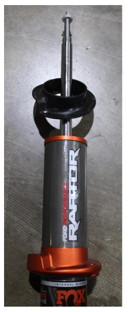
Remove Live valve wire clips in lower spring perch
