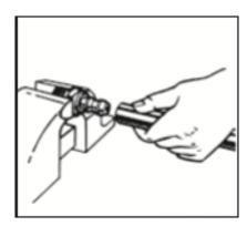
Step 2 – Secure fitting into Vise and begin pressing hose onto the fitting. Press the hose all the way on to the fitting until it is tight against the collar. You may use a heat gun to soften up the hose for easier installation.
