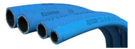
Howe Performance recommends using Eaton Aeroquip Low Pressure Push Lock style hose for all return lines. This is because the low pressure hose has a larger I.D. than high pressure hose and is less restrictive on the return line. It is similar to taking your thumb off the garden hose and letting the water free flow out. We use this in -8,-10 and -12 sizes.
