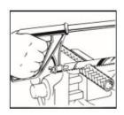
Step 1 – Cut hose square with a hack saw or cut off wheel
