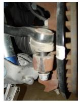
Stock Upper Control Arm to knuckle ball joint. Remove this using the same method as the OE stock Tie Rod.
